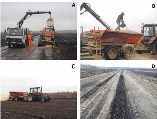
Figure 137. The process of wood ash dispersal. Photo: G. Spalva: A – Transportation and loading of wood ash; B – kMoisturising of wood ash; C – Dispersal of wood ash; D – Dispersed ash before its incorporation in the soil
